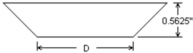
$$K_2 = \frac{0,577 * \pi * E * d}{\text{Ln} \left[ \frac{(1,15t + D - d) * (D + d)}{(1,15t + D + d) * (D - d)} \right]}$$
