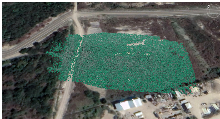
Figure 4.10: Sparse point cloud georeferenced seen from Google Earth.
