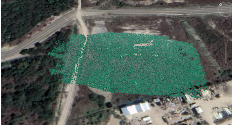
Fig. 7: Sparse point cloud georeferenced seen from Google Earth.
