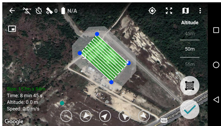
Figure 4.4: Screenshot of Altizure, the mobile application used to implement the flight strategy for image acquisition.
