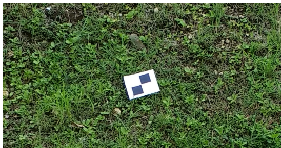
Figure 4.9: Target example used for easy GCP detection in the images.
