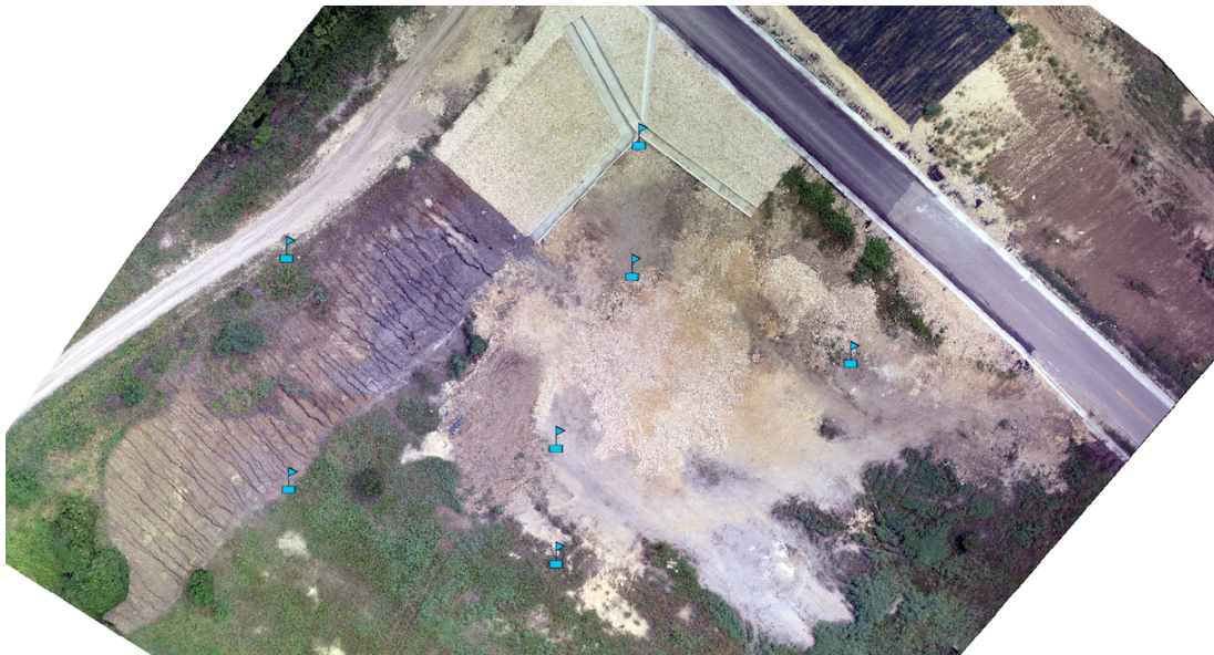
Figure 5.5: GCP network used in the validation process.
