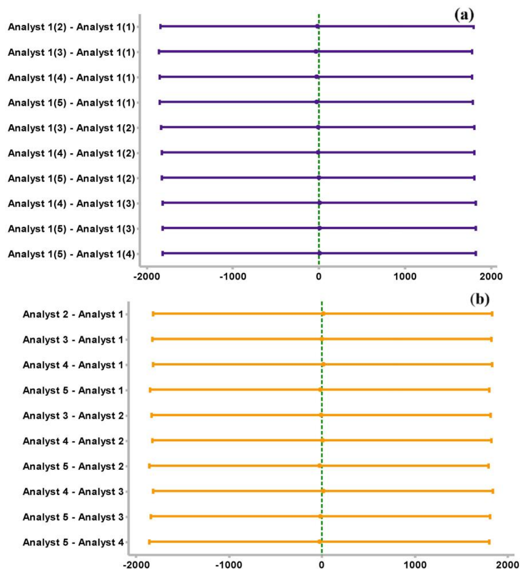
Figure 5. (a) Difference of means compared one to one for repeatability of the calibration curve. (b) Difference of means compared one to one for calibration reproducibility.
