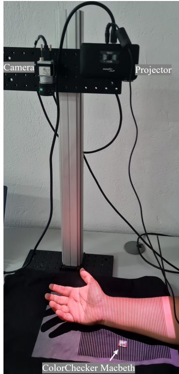
Fig 4 3D imaging setup composed of a camera, a projector and a Macbeth colorchecker.
