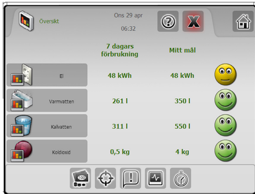
Fig. 5. TV-channel showing the energy consumption (for the last 7 days in this case, and individual targets) in the apartments of group IV [25].
