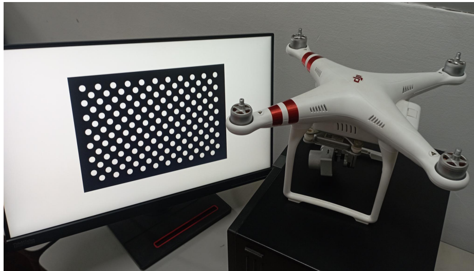
Figure 5. Camera Calibration setup using a 7x21 white circle asymmetric pattern and DJI Phantom 3 Professional drone.
