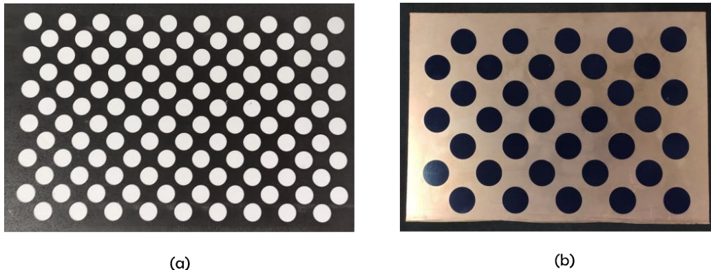
Figure 2: Targets used in calibration: (a) Structured light target, and (b) Target of the visible-thermal camera system.
