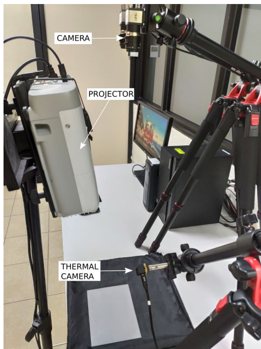
Figure 1: Multimodal structured light and thermal imaging system.
