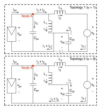
Figure 3. Topologies of the PV system based on the NEC boost converter.
