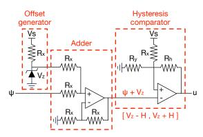
Figure 9. Switching circuit implementing the control law (51).
