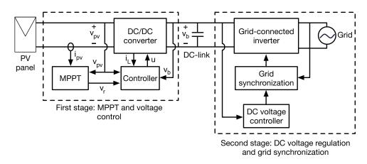
Figure 1. Structure of a PV microinverter with DC-link regulation and grid connection.
