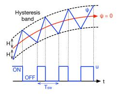
Figure 8. Hysteresis band to limit the switching frequency.
