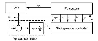
Figure 10. Complete control structure.
