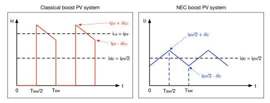
**Figure 5.** Waveforms of the output currents of classical boost and NEC boost PV systems (d = 0.5).
