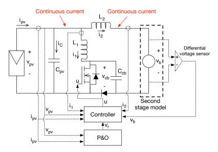
Figure 2. Circuital description of the PV system based on the NEC boost converter.
