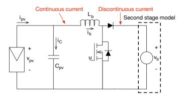
Figure 4. PV system based on the classical boost converter.
