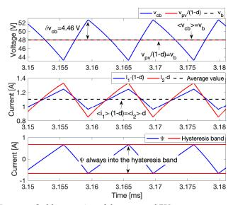
Figure 16. Stable operation of the proposed PV system.
