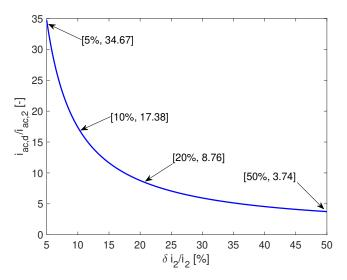
**Figure 6.** Comparison of the AC components introduced into the second stage by both the classical and NEC boost solutions (d = 0.5).
