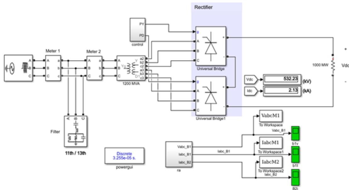
Figure 3. 12-pulse AC-DC converter circuit with filter.
