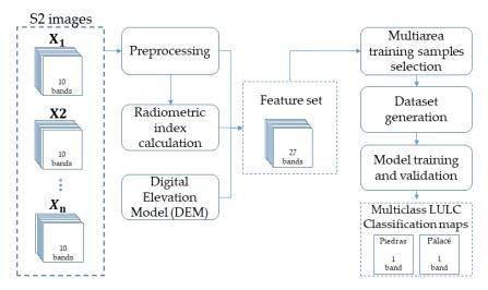
**Figure 2.** General block scheme of the proposed approach for LULC classification of Andean subbasins in Colombia.
