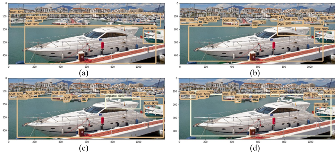
Figure 1. Performance of (a) SSD method using the inception, (b) R-FCN method using the Resnet101, (c) Faster R-CNN method using the Resnet101 and (d) Faster R-CNN method using the Inception and Resnet101.
