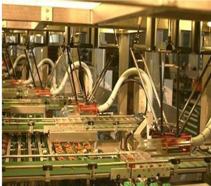
**Figura 1.8.** Demarex's Line-Placer installation for the packaging of pretzels in an industrial bakery (courtesy of Demarex)
