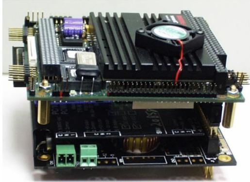
**Figura 3.33.** Tarjeta de control PC104.
