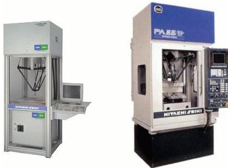
**Figura 1.10.** Hitachi Seiki's Delta robots for pick-and-place and drilling (courtesy of Hitachi Seiki).
