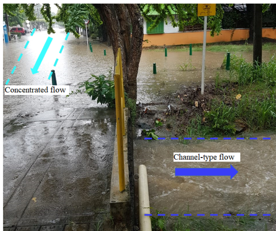
Figure 2. Identification of concentrated flow and channel flow in one of the small watersheds of the case study (city of Montería, Colombia).
